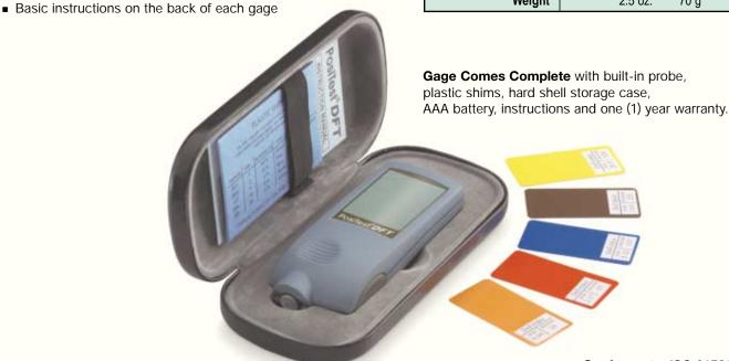
Conforms to: ISO 2178/2360/2808, prEN ISO 19840, ASTM B244/B499/B659/D1186/D7091-05/D1400/E376/G12, BS3900-C5, SSPC-PA2 and others. Certificate of Calibration traceable to NIST available.
