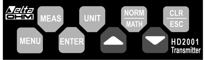
**MEAS** By repeatedly pressing this button the main variable displayed in the first line of the display can be selected. This function is cyclic: %RH >> Barometric Pressure >> Wind speed (for the HD2001.2 model) >> %RH...
