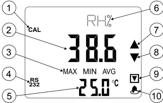
The display constantly shows the measurements of two values. While in the first line ② the value can be selected through the MEAS button, the second line ⑤ below always shows the temperature. During measurement, the first line ④ displays the unit of measurement of the main variable; inside the menu it provides information about the active item.
